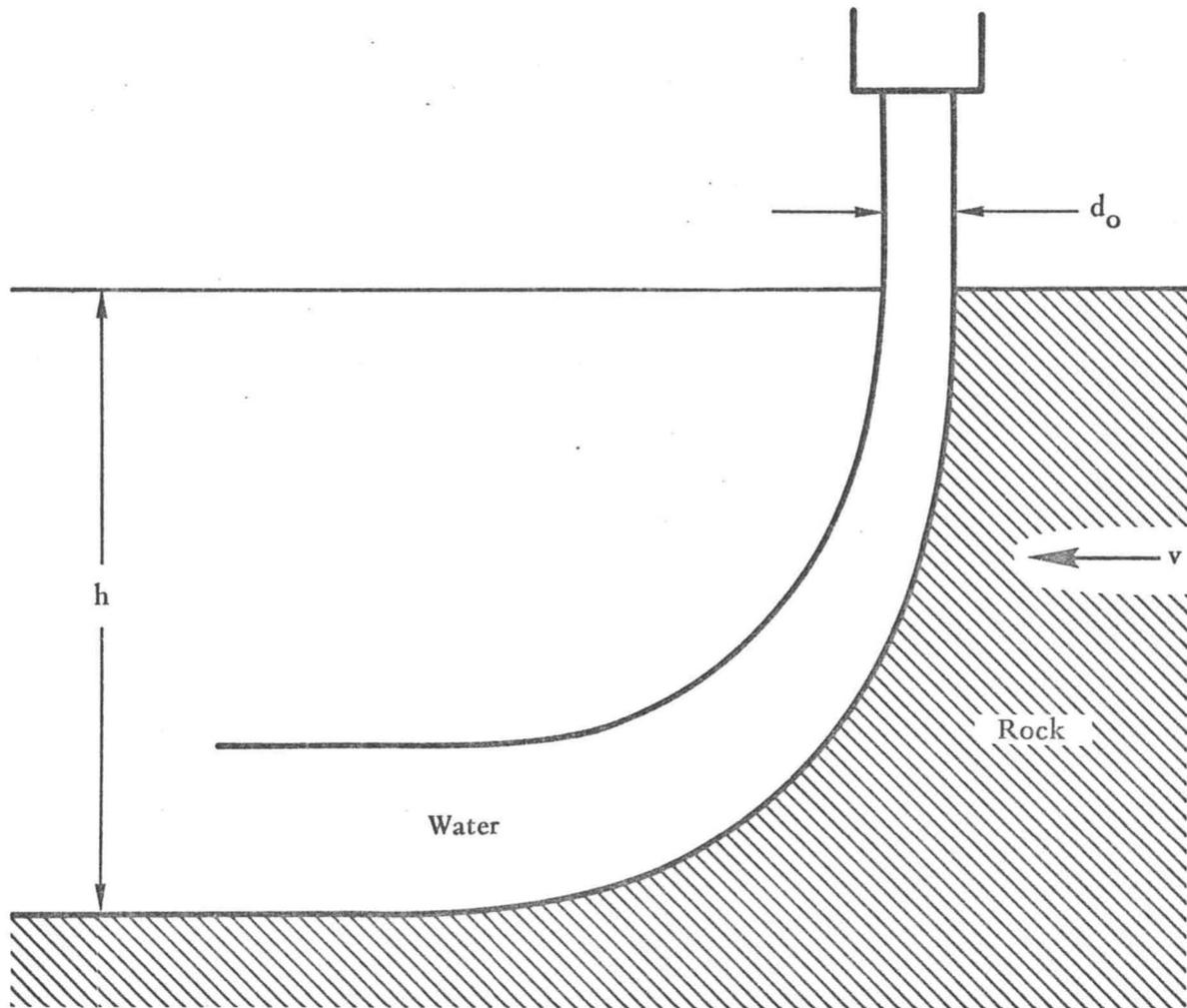
Figure 1. Cutting by a steady high-speed water jet.
